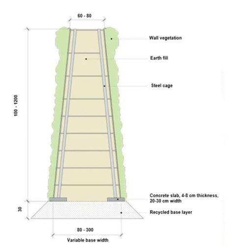
The easily connectable, enormously stable basket consists of carrier profiles, vertical needles and outdoor mats. The foundation is easy to make and fast to finish. All pourable floors may be used for the filling. Sharp curves, jumps in height or embankments are no problem for the R3. **Deviations from** standard profiles (a trapezoid with 60 centimeters crown width and 10% Angle on both sides) can often be realized without extra costs.
